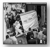
In this photograph, at least four men are struggling to maneuver the hard drive onto a truck. The 1956 IBM Model could hold 5 MB of storage which is about 6 images worth.
